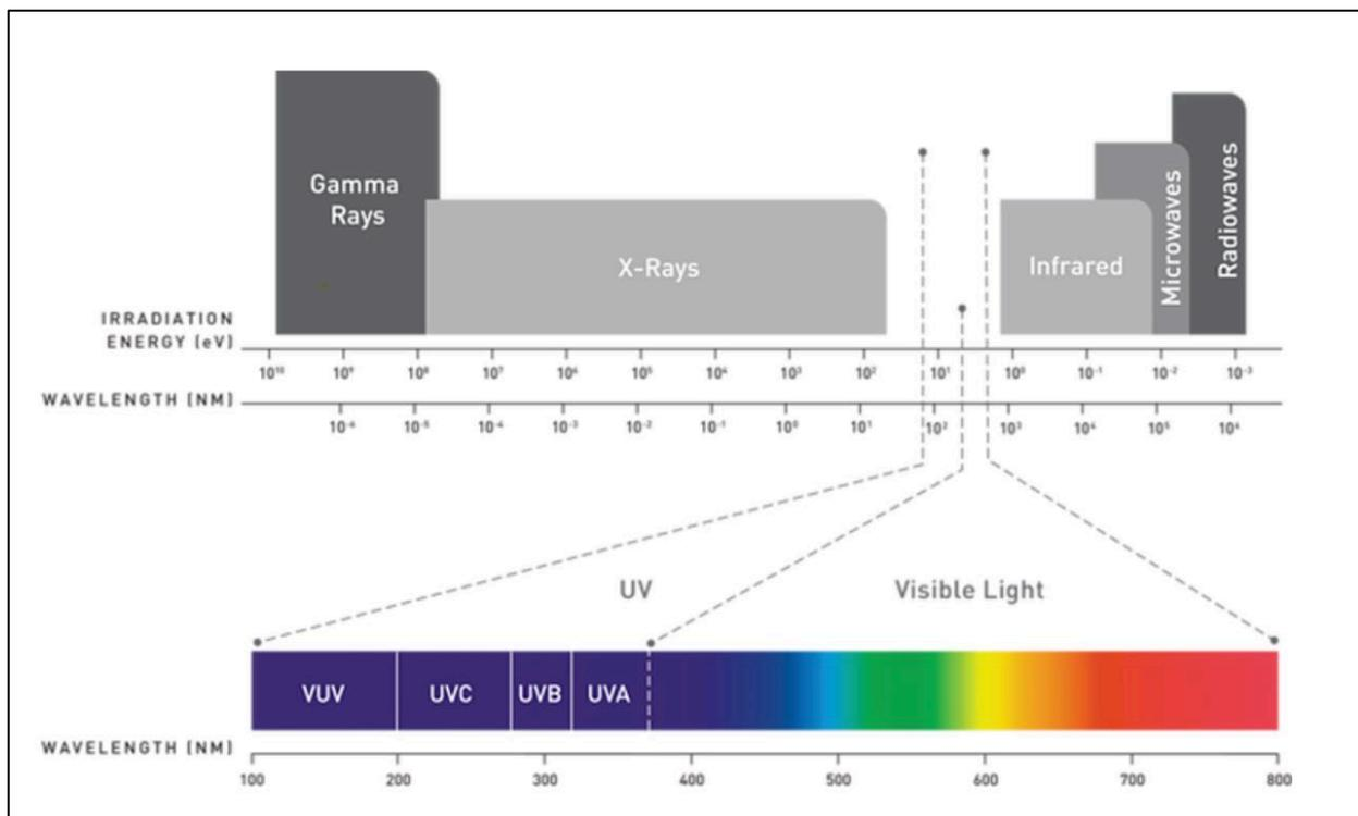
There are three ranges to UV light – UV-A, UV-B, UV-C and Vacuum-UV:
